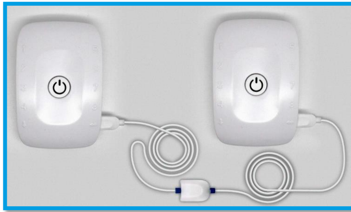
Figure 130: biosignalsplux devices connected with a sync-cable.
